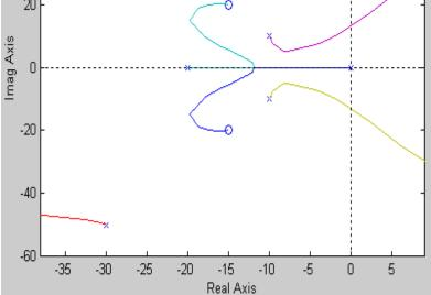
The root locus is a graphical procedure for determining the poles of a closed-loop system given the poles and zeros of a forward-loop system. Graphically, the locus is the set of paths in the complex plane traced by the closed-loop poles as the root locus gain is varied from zero to infinity.
