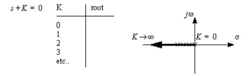
Note: because all of the roots for all values of K are real negative this system will always be stable, and it will always tend to have a damped response. The large the value of K, the more stable the system becomes.
