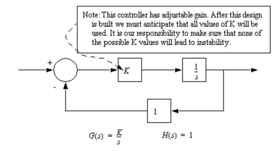
First, we must develop a transfer function for the entire control system.
