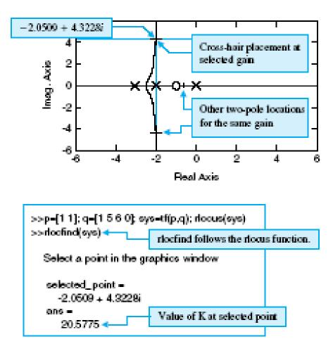
No matter what we pick K to be, the closed-loop system must always have n poles, where n is the number of poles of G(s).
