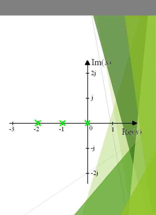
The loci on the real axis are to the left of an ODD number of REAL poles and REAL zeros of G(s)H(s)
